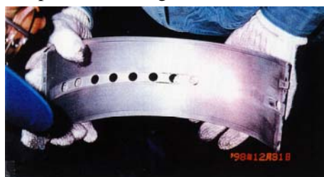
Fig.9 Crank Pin Metal of an Engine Equipped with the FHS, Fire Ring and the Kidney System
